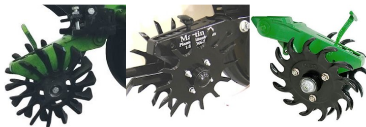
Figure 4 – Closing wheels used for the trial - from left to right - Yetter Paddle, Martin Spikes and Dawn Curvetine
